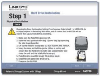
Physical Installation of the Second Hard Drive
