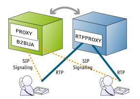
This server is installed next to the PortaSIP server running the SIP proxy and B2BUA. (Since fast and reliable connectivity between the PortaSIP server and the RTP proxy is important, they should be connected by the same Ethernet link.) The RTP proxy will be controlled by B2BUA, so that when a customer tries to make a phone call and proxying is required, B2BUA will give a command to open the ports, and the RTP stream will flow to the server running the RTP proxy.
