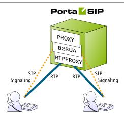
The RTP proxy does not perform any transcoding, and so requires a minimum amount of system resources for call processing. A PortaSIP server doing RTP proxying on an average PC server can support about 750 simultaneous calls.
