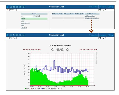
Defined in terms of connection threshold, the connection utilization graph shows the saturation of your connections, as well as the setup time and ASR.
