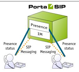
PortaSIP includes an advanced messaging module that enables online messaging, server-side message storage for offline users (so they can receive messages later), and the option of maintaining full message history on the server. The messaging module is implemented as an internal part of the PortaSIP proxy server, and enables communication between users by means of SIP MESSAGE packets.
