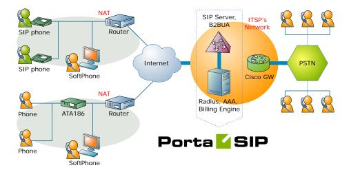
PortaSIP is a call control software package enabling service providers to build scalable, reliable VoIP networks. Based on the Session Initiation Protocol (SIP), PortaSIP provides a full array of call routing capabilities to maximize performance for both small and large packet voice networks.
