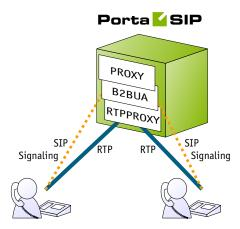
Voice traffic is quite different from other types of Internet traffic (e.g. web downloads), as it is very sensitive to packet delays. At any given moment, the system needs to transport packets at a constant speed and with minimum added delay. If a PortaSIP server is loaded with other tasks, this may become difficult. So now you have the option of installing the RTP proxy on a separate server.
