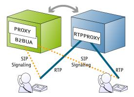
This server is installed next to the PortaSIP server running the SIP proxy and B2BUA. (Since fast and reliable connectivity between the PortaSIP server and the RTP proxy is important, they should be connected by the same Ethernet link.) The RTP proxy will be controlled by B2BUA, so that when a customer tries to make a phone call and proxying is required,
