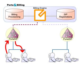
In this case, the call flow is exactly the same as in a situation where only one PortaSIP server is available (discussed earlier in the SIP  $UA \leftarrow SIP$  UA section).
