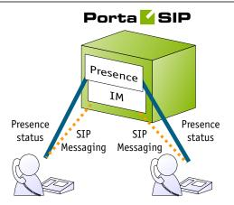
PortaSIP includes an advanced messaging module that enables online messaging, server-side message storage for offline users (so they can receive messages later), and the option of maintaining full message history on the server. The messaging module is implemented as an internal part of the PortaSIP proxy server, and enables communication between users by means of SIP MESSAGE packets.
