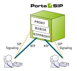
Voice traffic is quite different from other types of Internet traffic (e.g. web downloads), as it is very sensitive to packet delays. At any given moment, the system needs to transport packets at a constant speed and with minimum added delay. If a PortaSIP server is loaded with other tasks, this may become difficult. So now you have the option of installing the RTP proxy on a separate server.
